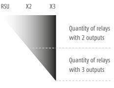
RSU 2223 = 2 relays with 2 outputs and 2 relays with 3 outputs
